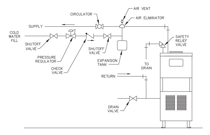
Figure 3.1: Supply and Return Piping
